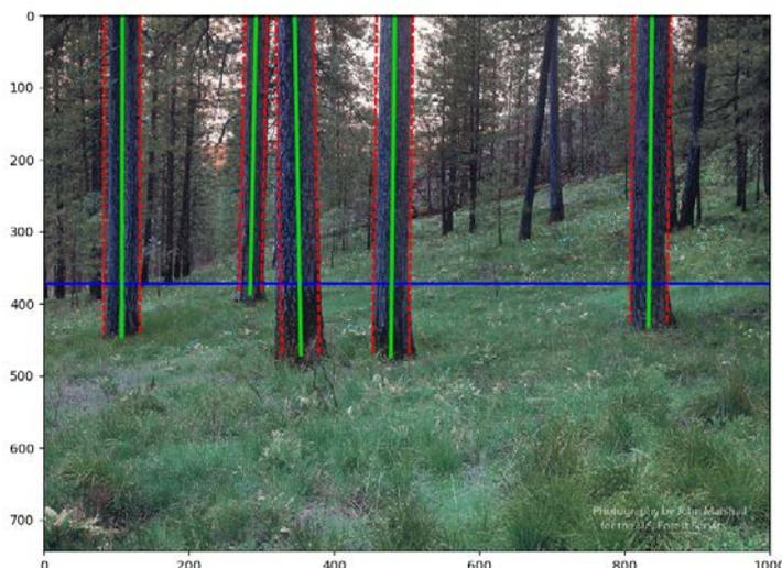
*A 3D machine vision technology developed to detect and measure tree characteristics real-time during thinning operations. (Credit: Lucas Wells, Oregon State University)*
